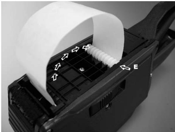
***Note that the backing material is place behind the two pins at the bottom-front (refer to arrows). In this way a correct printing is ensured.***
