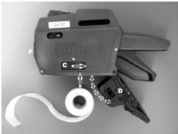
***Press both stop pins (C) in direction of arrow to open bottom (D). Insert new label roll as shown on figure.***
