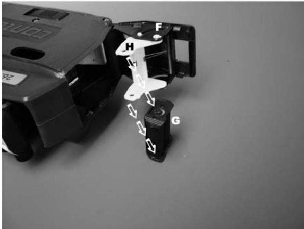
*Hold the knurled area of carriage (G) between thumb and index finger, spread the yellow swivel arm (H) until you can pull carriage with ink rollers out of the front (F).*
