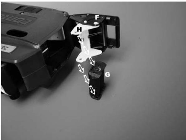
*Hold front plate (F) and yellow swivel arm with one hand. Take carriage at knurled area with the other hand and make it horizontally snap in (see direction of arrow)*
