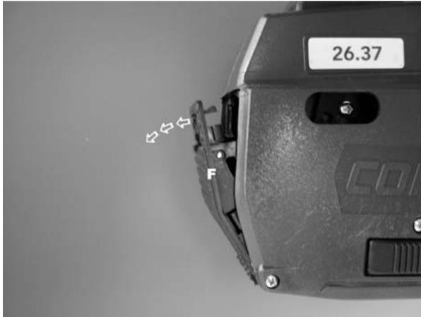
*Put the index finger into rectangular bore at front plate (F), support with thumb on housing and open front plate with index finger.*
