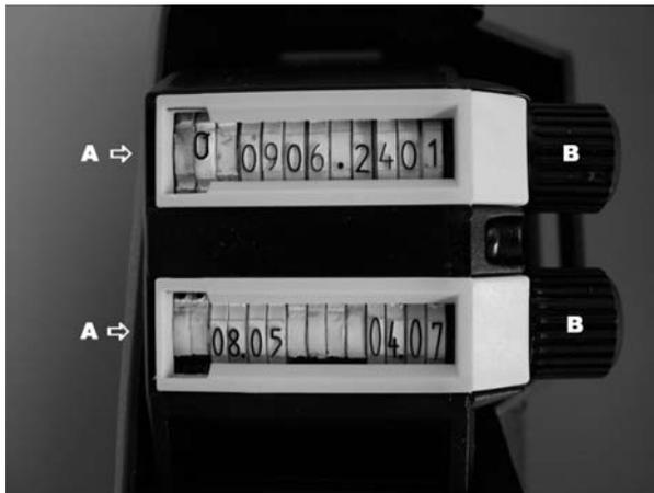
***Pull adjustment knob (B) to the desired position and turn knob to select character to be printed. (A) The 14. position on print band is always vacant ! IMPORTANT: Adjustment knob must be pressed in before operating to avoid damage to the print head.***
