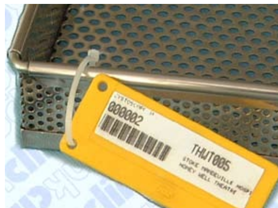
The tags may be written upon with non-toxic markers or labelled with bar codes as shown.
