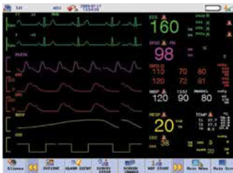
OxyCRG: Displays the interactive relationship between heart rate, respiration and oxygen on the same screen.
