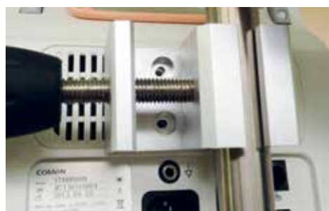
Correct Pole Mounting
